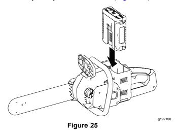
3. Push the battery pack into the battery cavity until the battery pack locks into place.
