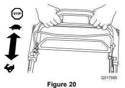
**Note:** Use the traction-assist handle in situations when you need more control than you have with the self-propel drive alone.
