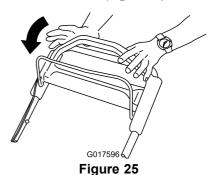
**Important:** When you release the blade-control bar, the blades should stop within 3 seconds. If they do not stop properly, stop using your machine immediately and contact an Authorized Service Dealer.
